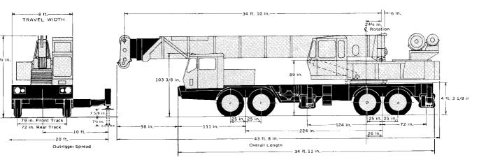
TURNING RADIUS -– 39 ft. 4 in. GROUND CLEARANCE — 14 in.
